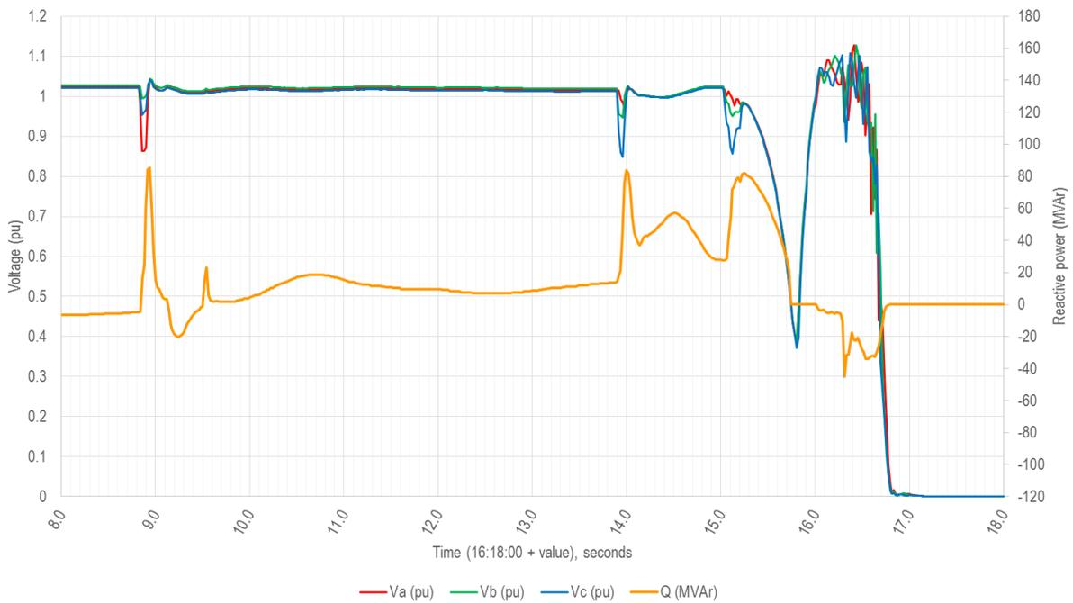
**Figure 70 Three-phase voltages and MVar injection by Para SVC2**
